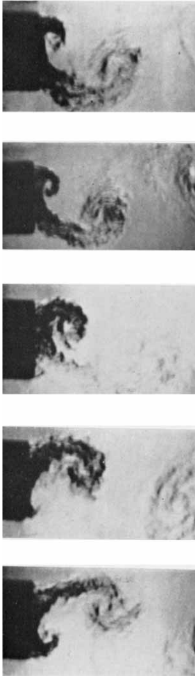
FIGURE 6. Schlieren photographs of vortex shedding from Archibald.
